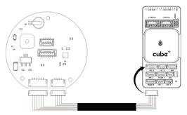
For Cube Orange Plus → plug the other end into the 8-pin GPS1 Port
