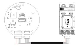
For Pixhawk → plug the other end into the 10-pin GPS Module Port
