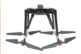
The axl 30L Drone Kit is an Advanced Foldable version of axl 30, which pairs our lightweight carbon-fiber airframe with the necessary propulsion components (Motors, ESCs, and Propellers) so you get advanced performance without the hassle of sourcing parts.
