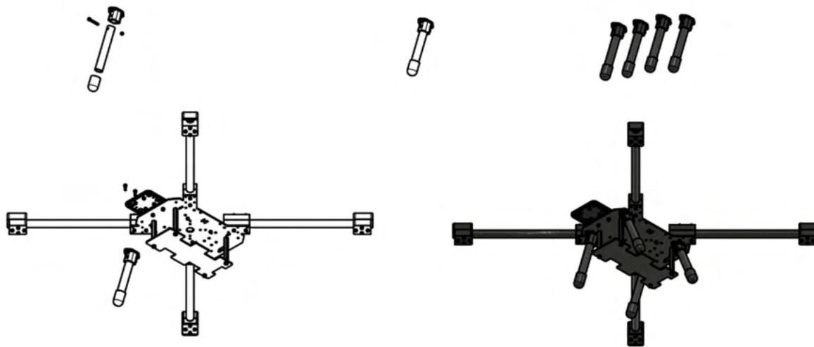
The landing gear is attached to the bottom panel using a 10mm long M3 Allen bolt and nut.
